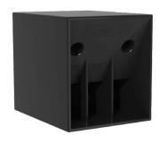
The DS-18S is an extremelly high power subwoofer cabinet providing exceptional low frequency reinforcement for the DS-12. It uses one 18" (4" DUO voice coil) transducer with aluminium demodulating ring in direct radiation bass reflex configuration. Manufactured as standard with premium birch plywood and finished with polyurea coating it can also be manufactured in any colour or finish to compliment any install design.
