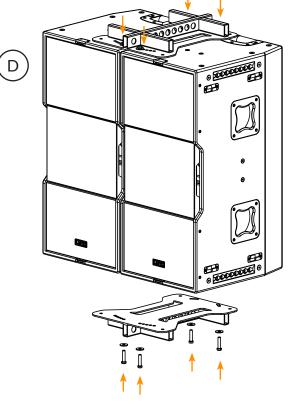
NOTE: Each hole has a degree position, as shown in the picture above. Make sure to insert the screws in the right holes to obtein the desired angulation.
