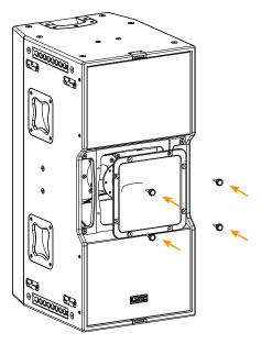
• Place the cabinet grill back into the former position. Make sure that the cabinet grill is properly fixed with the magnets.
