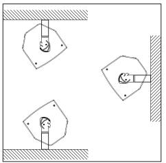
The first thing to do is to fix the UBR support in the place required (ceiling, wall, floor, etc).
