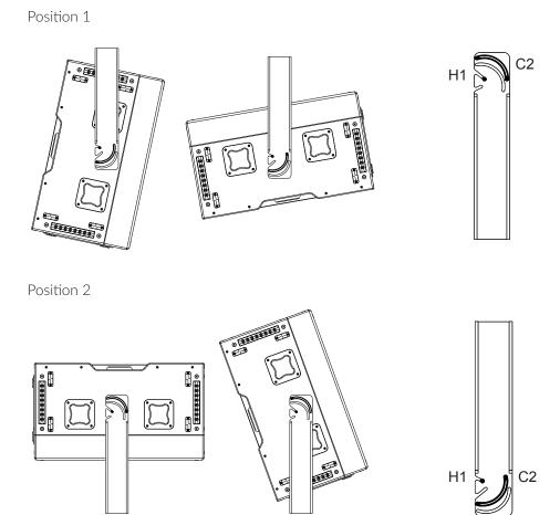
If you choose Position 1 or 2 you will have to insert two special fixing screws into the cabinet (one per side) before installing the enclosure. So firstly, take 2 of the fixing screws provided and insert them into your cabinet. Where? Have a look.
