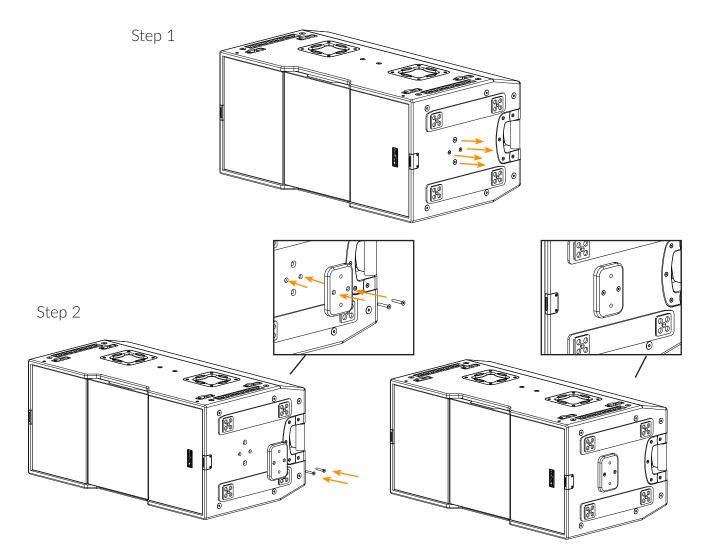
Once this is done, the U bracket for horizontal mounting can be correctly attached.
