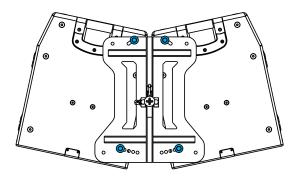
NOTE: The start position will be 0 degrees. The angulation can open up to 12 degrees. Each point will add 3 degrees of angulation.
