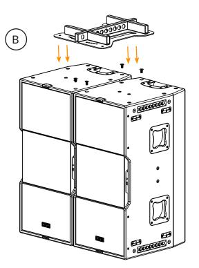
• Use the screws given in the support kit to secure the frame to both cabinets with the desired angulation, as shown in Figure C.
