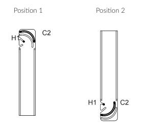
Now you have to use the appropriate curve groove of the UBR support in order to slide the other fixing screw per side and orientate the cabinet.
