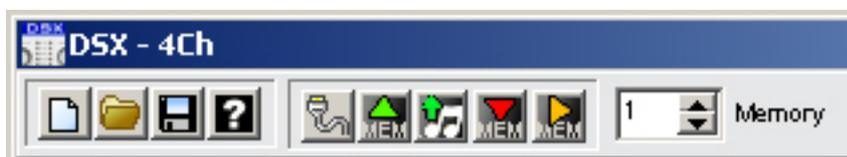
Use the button **Write to the Processor** to save into the selected memory. While establishing connection **Communications** screen appears, showing Info of the status of the communication (initialization, checks, communications and end of this one) and the progress bar shows the percentage of the entire transmission.
