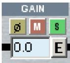
**Gain:** Pressing the "E" button, you will access the **Main Gains** window. From here you will be able to adjust the Gain on each input and output. You can also **Mute**, invert the **Polarity** or activate the "Solo" mode. You are also able to do all this from the **Main Window**.
