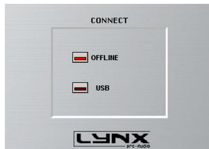
Connect the cable provided to a free USB port and select the mode to connect. If the communication is successful, communication screen will shortly appear giving way to the main screen of the software with the framework of the DSX.
