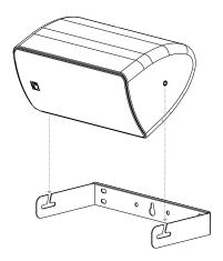
How to use it? The first thing to do is to fix the U bracket in the place required (ceiling, wall, floor, etc).
