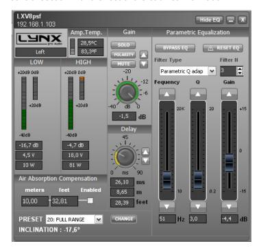
You can use up to 6 filters per way, totally configurable, which can be chosen between adaptable or constant Q, All Pass, Band Pass, Notch, HP Q, LP Q or High and Low Shelvs provinding flexibility.
